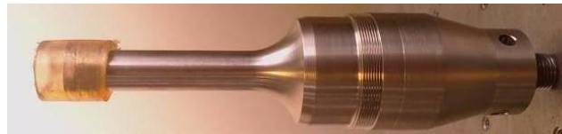
Figure 8 – Photo of the horn + tube
